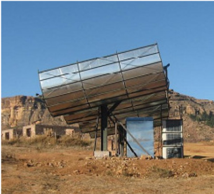
Solar ORC in field trials in Lesotho, southern Africa 2007 (Solar Turbine Group)
